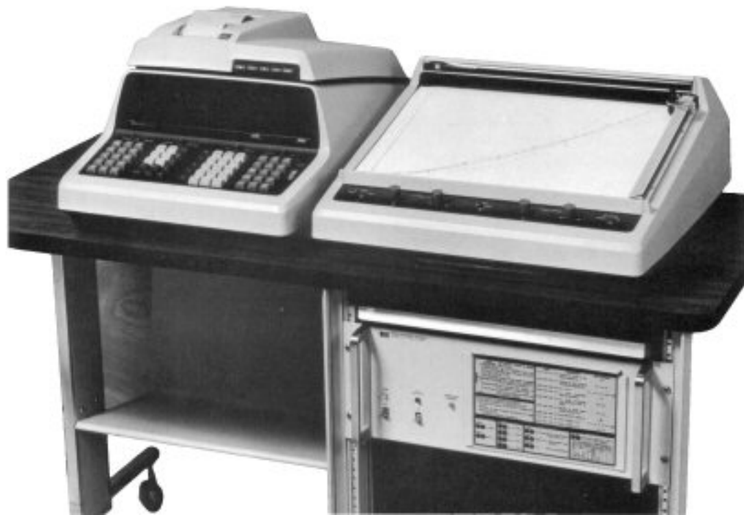
The HP 9100A had a difficult-to-design-to interface, but that didn't prevent HP engineers from developing several peripheral devices for the calculator, including the HP 9120A printer, HP 9125A plotter, and HP 9101A extended memory shown here. Photo courtesy Hewlett-Packard Company
